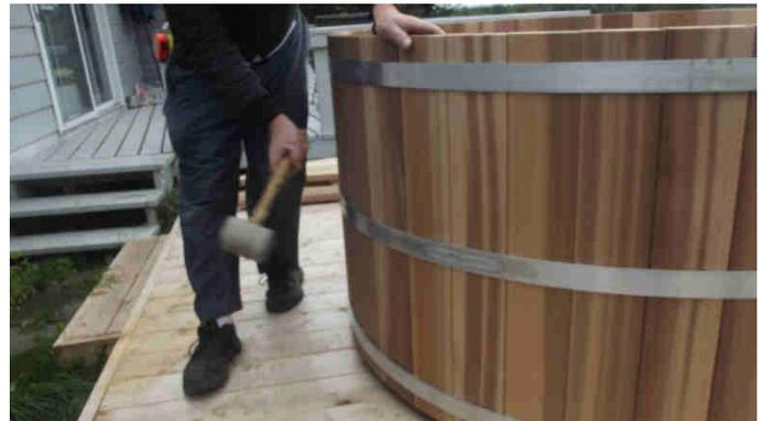
Fig. 9.2 Hitting straps hard all around while tightening.
