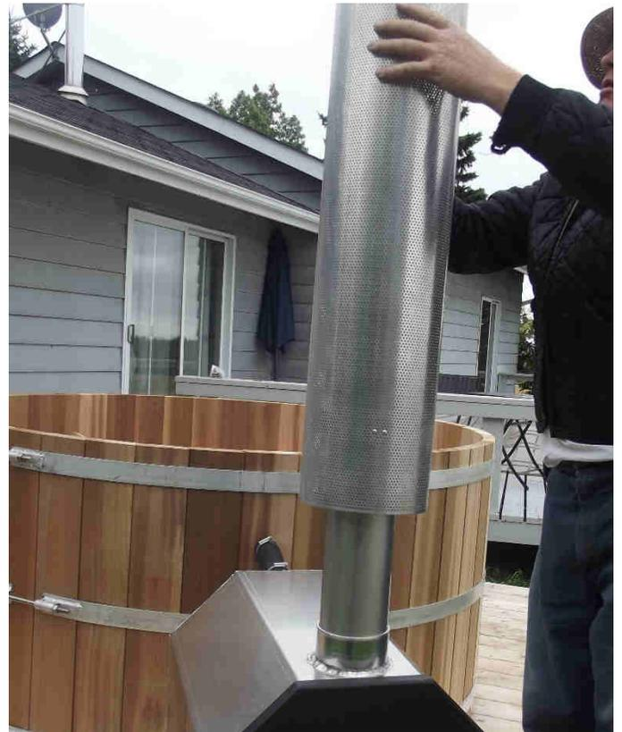
*Fig. 10.2.3 Assembling the heater stack.*
